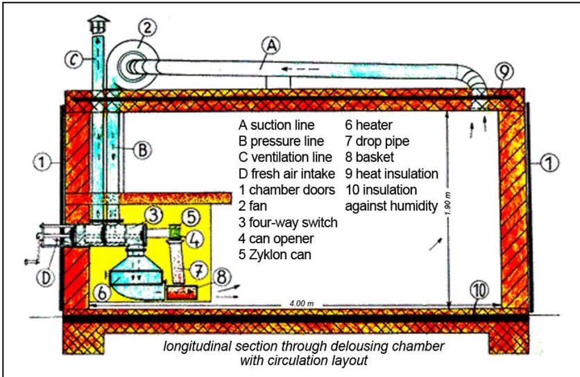
**Fig. 4:** DEGESCH delousing chamber with circulation feature.<sup>52</sup> This design was developed in the late 1930s / early 1940s and became a standard in Germany during the war. It was, however, not installed in all concentration camps, which were frequently equipped with makeshift delousing chambers.
