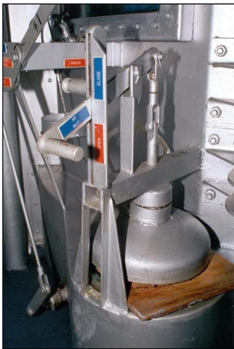
**Fig. 98:** Closeup of fresh-air intake of gas chamber.
