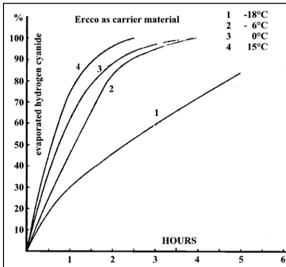
**Graph 2:** Evaporation rate of hydrogen cyanide from the Erco carrier material (gypsum with some starch) at various temperatures and fine distribution, according to R. Irmischer/DEGESCH 1942.<sup>182</sup>
