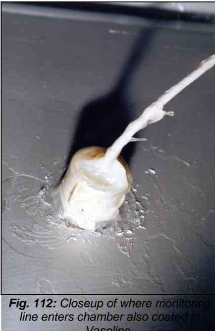
**Fig. 112:** Closeup of where monitoring line enters chamber also coated in Vaseline.
