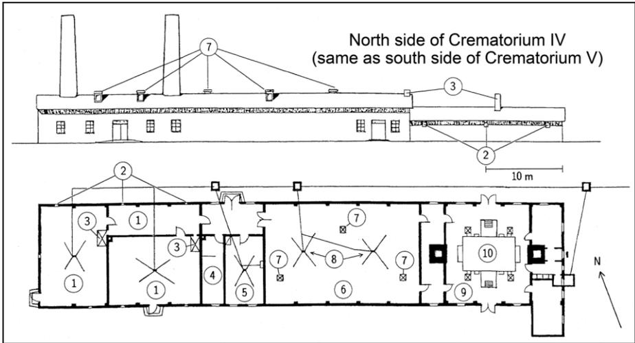
**Fig. 8:** North elevation (above) and ground plan (below) of crematorium IV and/or V (mirror image) in Auschwitz II/Birkenau camp.<sup>159</sup>
