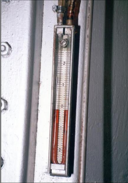
**Fig. 110:** Manometer to monitor relative gas chamber pressure.
