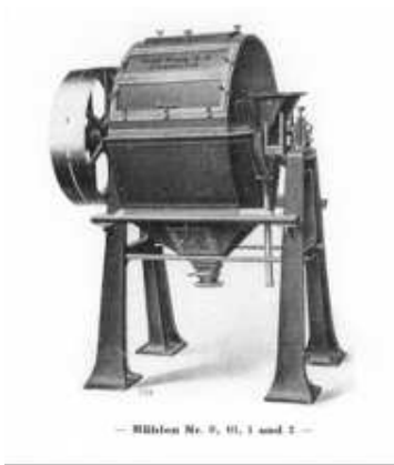
Fig. 11: According to a Krupp-Gruson brochure of 1915 the four light ball mills (Types nos. 0, 01, 1 and 2) looked practically identical. Source: Company brochure [29]
