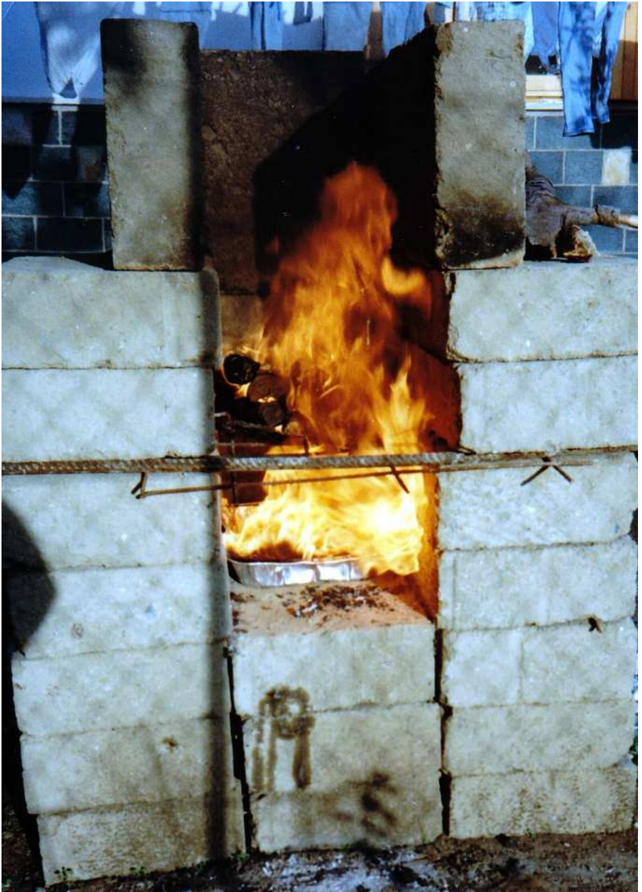
PHOTOGRAPH 7: Lard combustion experiment with pan below the combustion grid.
