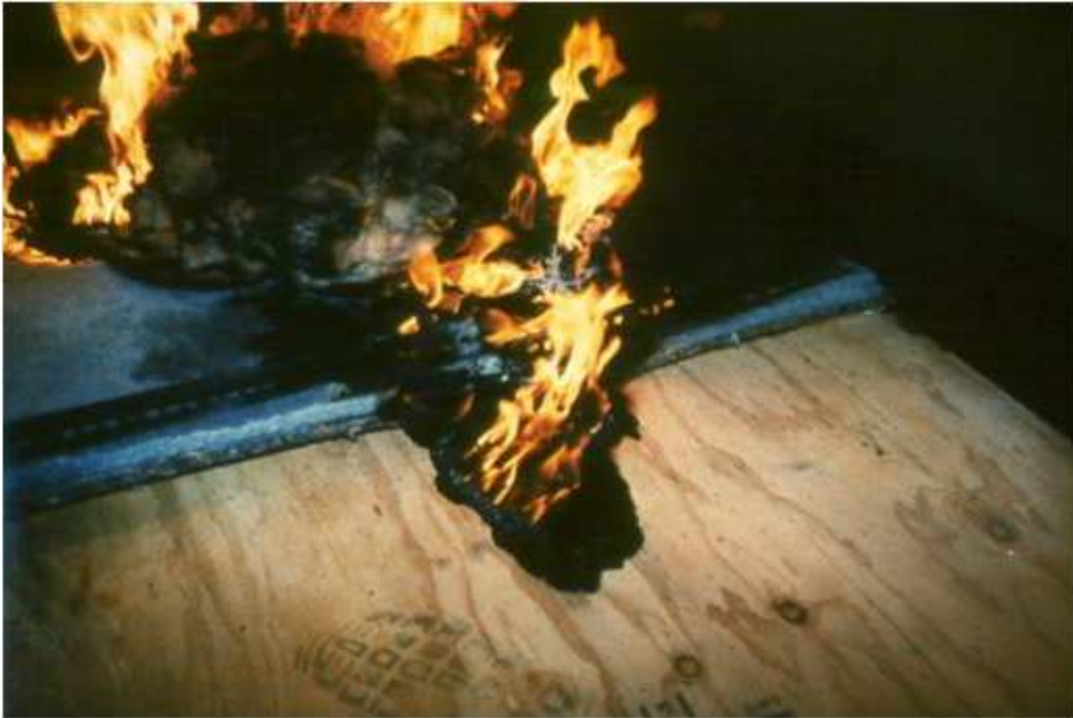
PHOTOGRAPH 4: Fat burning at one single limited point within a pit of liquid fat (Wick Principle). From: J. DeHaan and E. Pope, Combustion Properties of Human and Large Animal Remains [34]
